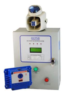
The Acme Quadset Refrigerant Gas Monitor is designed to detect refrigerant leaks in enclosed areas. The Monitor utilizes a sophisticated NDIR sensor specific to any one of the commercially available refrigerants. It can monitor over a range of 0-1000ppm with a resolution threshold as low as 1ppm.
